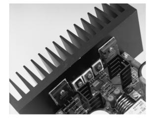
Fig. 4. Good thermal coupling between the transistors and the heat sink ensures a long life of the devices.
