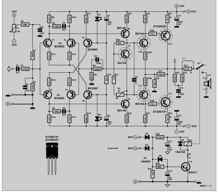
Fig. 1. Circuit diagram of the upgraded (IGBT) amplifier.
